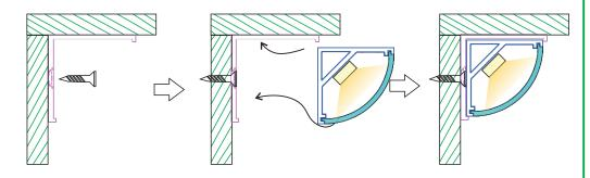
2, "Walk" along the wall in various directions. Support Straight Connection, L Connection.
