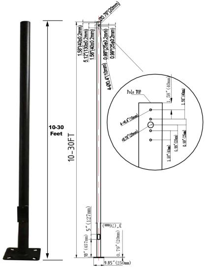
The WISDOM Series Round Steel poles are built from high strength Steel Round tube and are available side drilled for arm mounted area lighting luminaires or with tenon mounts for flood and post top luminaires. Typical area lighting applications include retail centers, industrial parks, schools and universities, public transit and airports, office buildings and medical facilities. Mounting heights of 10 to 30 feet can be used based on selected luminaire application.
