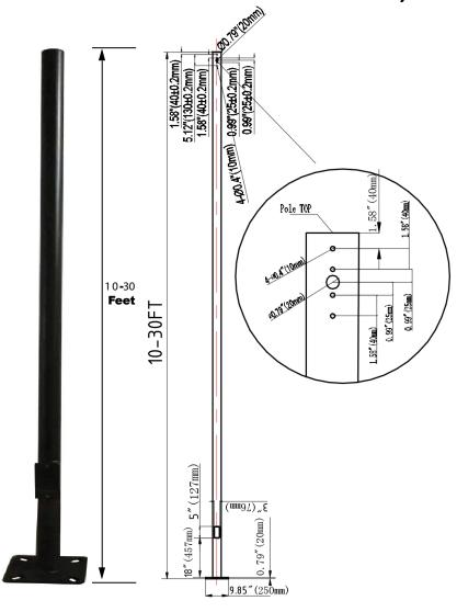
The WISDOM Series Round aluminum poles are built from high strength aluminum Round tube and are available side drilled for arm mounted area lighting luminaires or with tenon mounts for flood and post top luminaires. Typical area lighting applications include retail centers, industrial parks, schools and universities, public transit and airports, office buildings and medical facilities. Mounting heights of 10 to 30 feet can be used based on selected luminaire application.
