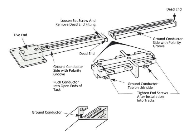
Remove dead ends from tracks, align ground tab to proper side of the track to match polarity, insert connector and tighten screw.
