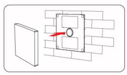
4. Put the rotating switch on the front of holder.
