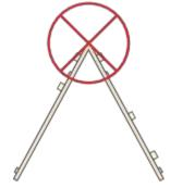
Bending strips sheets or sections at sharp angles will damage circuit traces and void warranty
