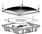
2. Connect the wires threaded from conduit and Canopy, Black wire for Line, White for Neutral, Green/Yellow Green for Ground.
