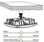
3. Screw the Conduit into the hole on top of Canopy light. Installation done.
