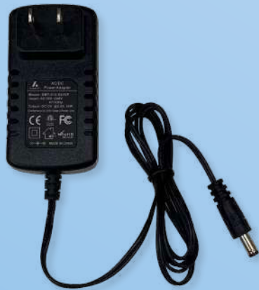
24W NON-DIMMABLE PWR-PLG-12V-24W-ID-G2 PWR-PLG-24V-24W-ID-G2 Rated for indoor use only (IP20). Input Voltage 100~240VAC Output Voltage 12VDC, 24VDC
