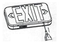
2. Knockout in back of mounting plate and push wires through the hole.
