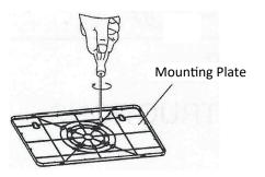
3. Securely attach mounting plate to J-box (not provided).
