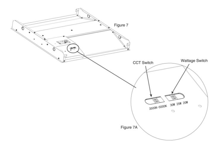
The end users may adjust the color temperature and lumen output respectively by the two DIP switch buttons integrated into the driver. Each DIP switch is accommodated with 3 options (left, middle and right), corresponding to 3 color temperatures and 3 powers respectively, which can perform the desired color temperature and lumen output combination.
