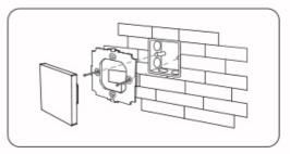
Fix the controller base on the bottom case with screw.
