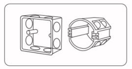
Install the bottom case into the wall: Above are the standard bottom cases.
