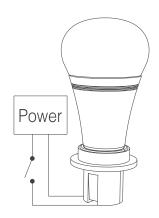
Switch off power to the device, after 10 seconds switch power back on
