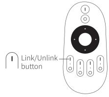
As soon as the light has power, and while it is flashing, quickly press the "Zone ON" button 5 times within 3 seconds. Un-linking must be done with the same Zone as linked to.
