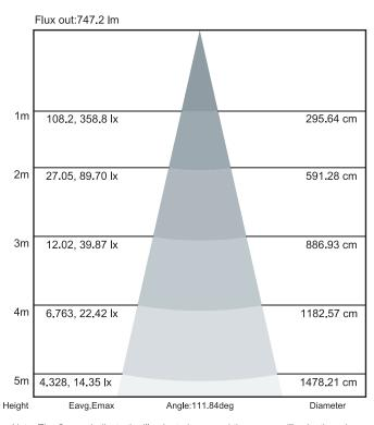
Note: The Curves indicate the illuminated area and the average illumination when the luminaire is at different distances.
