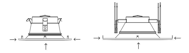
3. Flatten the four clamps to secure the trim to the fixture.
