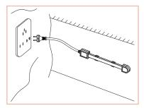
Fix the strip into clip, connect the input plug to the electric power, then it can be illuminated
