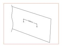
Position the screw hole in each 1 meter interval, for the place where the strip should be installed.
