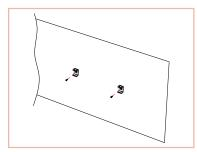
Fix the clip on the screw hole and lock it.
